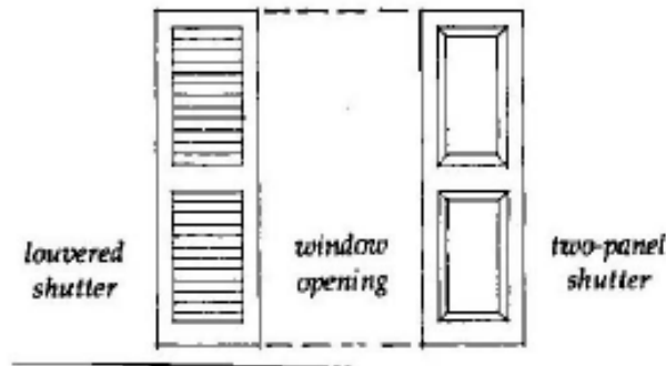
Figure 6.1 - Illustration of shutter styles and relationship to window opening.
